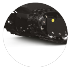
C — Tendicingolo a grasso Greased track tensioner
